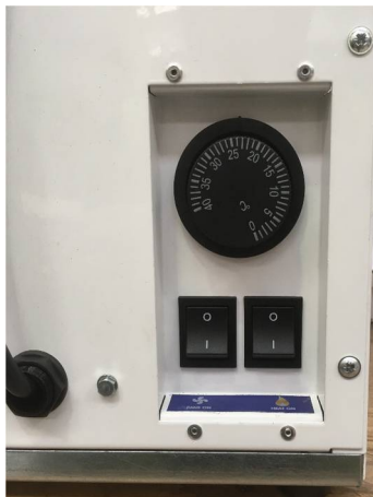
Recessed tamper proof controls at rear of machine
